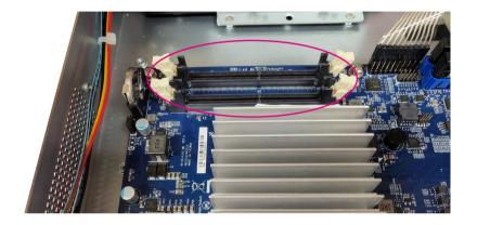
2. Release the locks on the DIMM memory sockets. Insert the modules into the sockets at a 90 degree angle. Apply firm even pressure to each end of the modules until they slip into the sockets.
